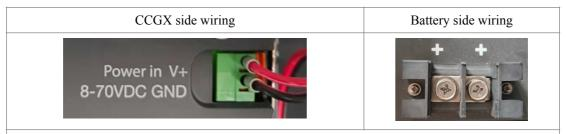
Note: Please connect the positive pole of the GX controller power cord to the positive part of the battery, and connect the negative part of the battery to the negative pole of the GX controller power cord.
